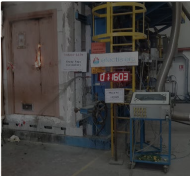
After 1 hour 16 minutes, the door starts to burn.
